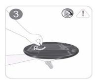
Turn the connecting screw at the bottom of the stand fully so that it is completely fixed.
